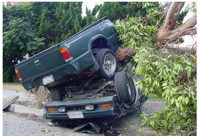
This vehicle, a Mazda pick-up, impacted the tree on the driver's side while upside down. It then wrapped around the tree as the tree fell. The Mazda was broken in half right behind the cab.
